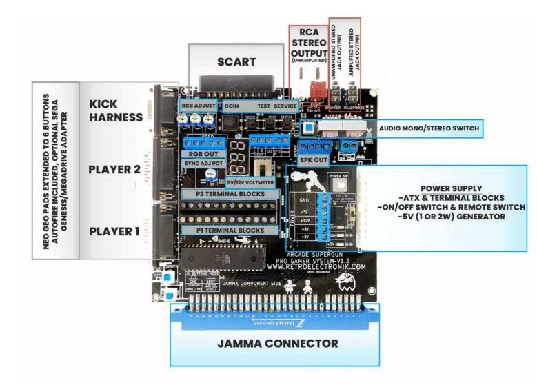
We designed the pro gamer to be as simple as possible without soldering or jumpers. Configuration can be done using 13 switches:
